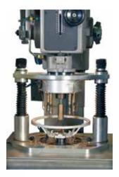
Multi-spindle headstock drilling detail of car handwheels.
