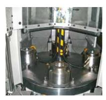
4 Positions rotating table for circular drill battery with syncronized hydraulic clamping tools.
