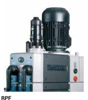
Automatic tapping cycle by lead screw system with brake motor for spindle reverse.
