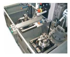
Hydraulic self-centering clamping tools for automotion hinge.
