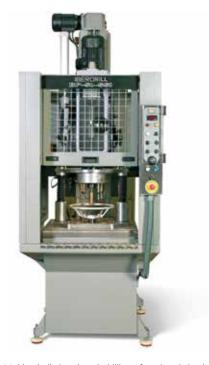
Multi-spindle headstock drilling of car handwheels, under strict technical and security standards.
